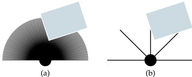
Fig. 1. (a) A typical laser rangefinder scan arrangement, providing 180 degrees of dense coverage in one-degree increments; (b) A sparse sensor, which gives only five range readings in a single scan.
